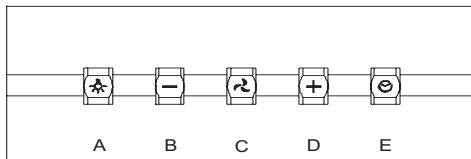
**A:** ON/OFF light switch: the hood light turns on or off when the button is pressed.
